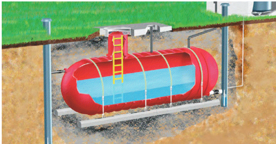
Figure 14: Fibreglass Water Tank
